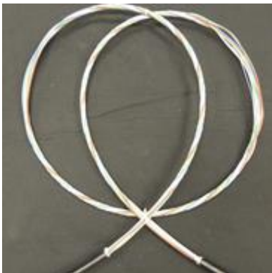
Cable with 178 cm (70 in) of jacket removed for mid-span splicing
